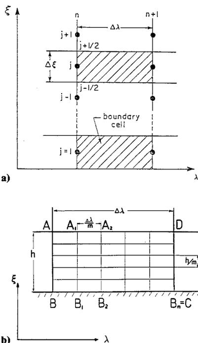
Fig. 1 Generalized Lagrangian coordinates  $(\lambda, \xi)$ : a) computational mesh; b) boundary subcells.
