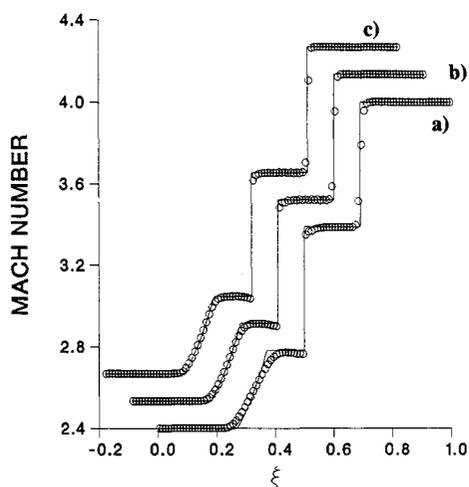
Fig. 2 Solution of steady Riemann problem for supersonic flow (Mach number distribution at  $\lambda = 0.5$ ): comparison of schemes. Symbols, computation; solid lines, exact solution: a) first-order Godunov; b) TVD; c) ENO.
