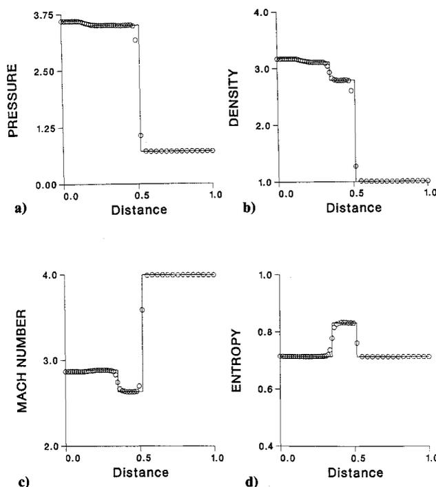
Fig. 4 Distributions of flow properties along a Lagrangian distance line ( $\lambda = 1.15$ ): a) pressure; b) density; c) Mach number; d) entropy.
