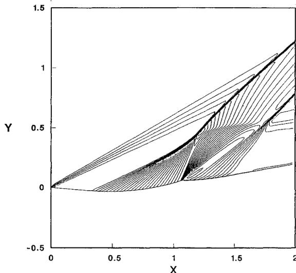
Fig. 8 Supersonic flow around a concave profile ( $M_\infty = 1.87$ ); Mach number contours.
