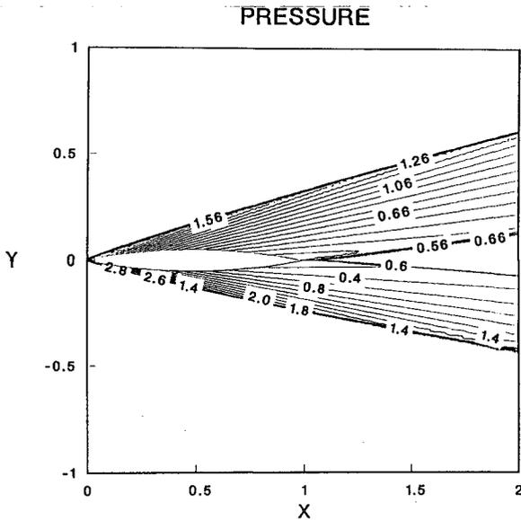
**Fig. 5 Steady hypersonic flow around a symmetric circular arc airfoil. Pressure contours (upper,  $M_\infty = 5.0$ ; lower,  $M_\infty = 8.0$ ).**
