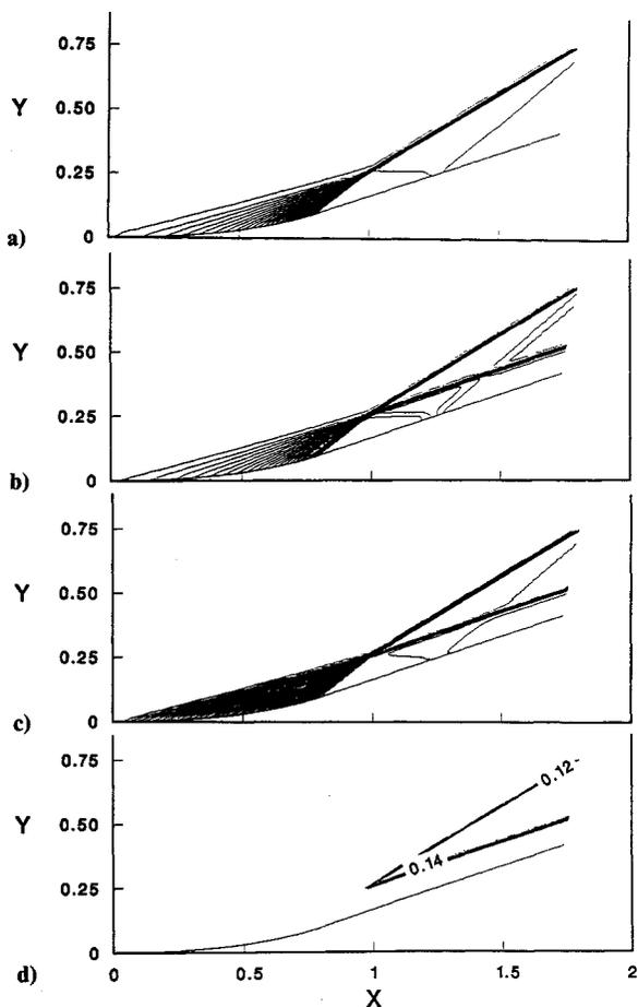
Fig. 3 Sudden formation of oblique shock wave of finite strength ( $M_\infty = 4.0$ ,  $M_1 = 2.867$ ); second-order TVD solution: a) pressure contours; b) density contours; c) Mach number contours; d) entropy contours.
