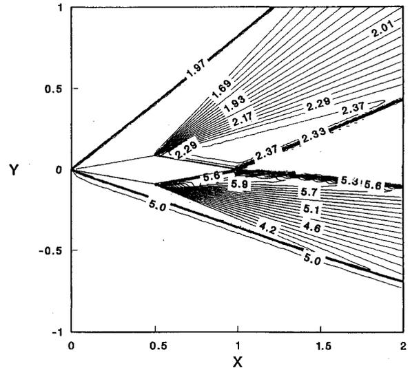
**Fig. 6 Steady supersonic flow around a double-wedge airfoil. Mach number contours (upper,  $M_\infty = 2.0$ ; lower,  $M_\infty = 5.0$ ).**
